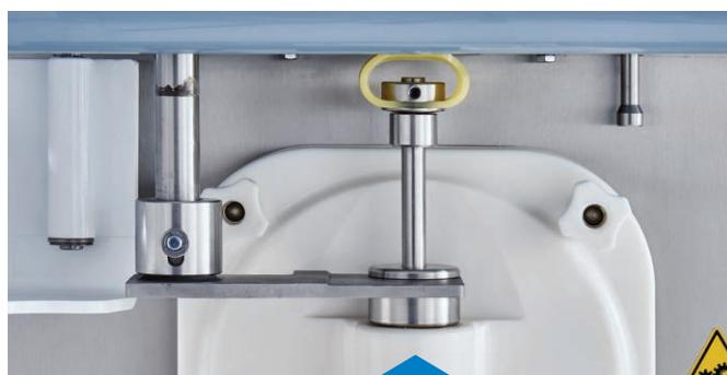
**Automatic delivery closure (only for K Shake models).** This machine is equipped with a portion control. The system delivers the correct portion required, regardless of the size of the cup.
