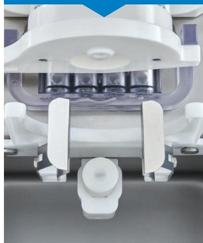
**Protective casing of the actuator (only for K Shake models)** dedicated for automatic production. Prevents any interference from the operator.
