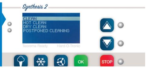
The delayed cleaning program guarantees hygiene by controlling the temperature of the cylinder once the gelato has been extracted. So immediate washing of the machine is not necessary in the event of prolonged work stoppages.
