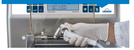
The **delayed cleaning program** guarantees hygienic by controlling the temperature of the cylinder once the gelato has been extracted. So immediate washing of the machine is not necessary in the event of prolonged work stoppages.
