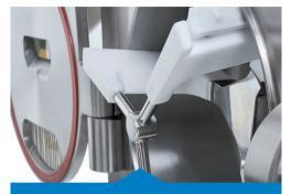
The beater's POM blades – impenetrable by the hot and cold – facilitate the **complete extraction of the gelato and creams**. It has self-adjusting scraper blades to maintain the cylinder clean and efficient.
