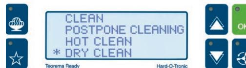
Once washing has been completed, all humidity can be eliminated from the cylinder with the **drying program**, essential before tempering chocolate.
