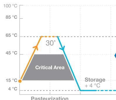
With the automatic **self-pasteurization (only for Super Tre AV EVO models)** system you can choose when to wash the machine up to a maximum interval of 42 days. As a further guarantee of hygienic safety, if the operator does not perform the complete cleaning at the end of the set days, the machine goes into automatic block.
