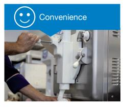
All commands remain accessible when the hopper cover is open so that the operator can start production while addina mix.
