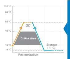
With the automatic self-pasteurization system you can choose when to wash the machine up to a maximum interval of 42 days. As a further guarantee of hygienic safety, if the operator does not perform the complete cleaning at the end of the set days, the machine goes into automatic block.
